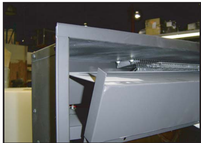
Fig. 5 Hold both sides and pull gently forward and down.
