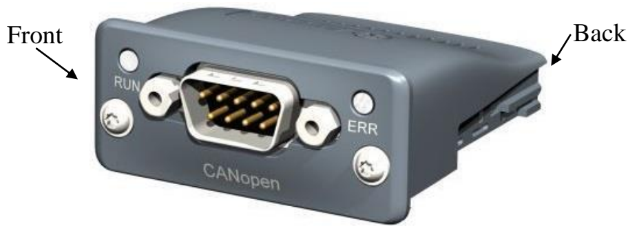
Figure 8 - ABCC module with CANopen interface [12]
