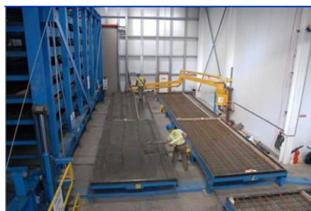
Figure 2 - CompactRIO system used to lift and control a concrete tray with high accuracy
