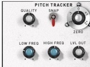
This module extracts the pitch of the input signal. The resulting pitch signal can be applied to the oscillators, but it can also be used to modulate any other modules via the connection matrix.
