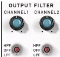
The two knobs set the cutoff frequency of the filters and the switch is selecting the type, high-pass or low-pass.
