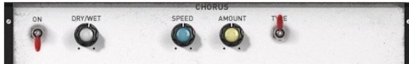
**DRY/WET:** Sets the mix level between the initial signal and the processed signal
