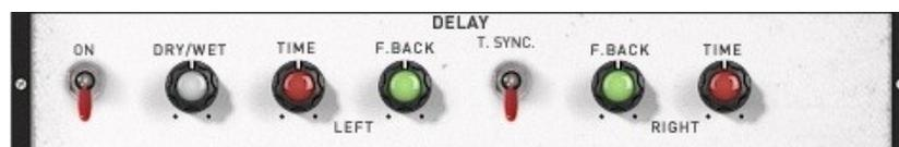
**DRY/WET:** Sets the mix level between the initial signal and the processed signal
