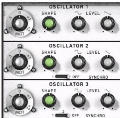
Three oscillators are available. The first one is outputting a sine wave and a saw, with independent level. The Shape knob allows to change the sine wave form and to add a new pulse to the saw.
