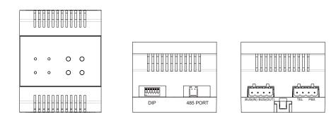
DIP switches, DIP settings refer to 3. 485 connection port, used to update the software for TPS. 485 PORT: Input port, connect to power supply. BUS(IN): Output port, connect to Monitor. BUS(OUT): Connect to the telephone. Connect to the telephone network.
