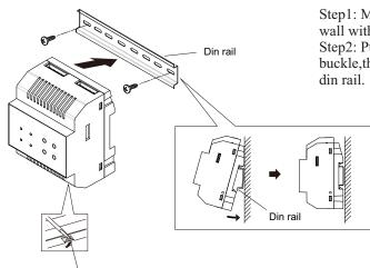
Step1: Mount the din rail to the wall with screws ; Step2: Pull down the mounting buckle,then hang the unit on din rail.
