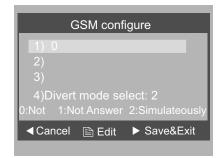
Maximum 3 telephone numbers can be set,Use ▲ /▼ Button to move upward / downward to select the item,then press the MENU button to edit.Use ▲ / ▼ Button to increase / decrease the value,and use ▶ button to input next digital,use ▶ button to ◀ button to cancel the input. press the MENU button again to finish the edit operation.
