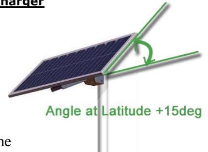
Recommended Solar Panel Angle
