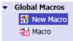
Figure 5-7: Identifying macro components containing errors
