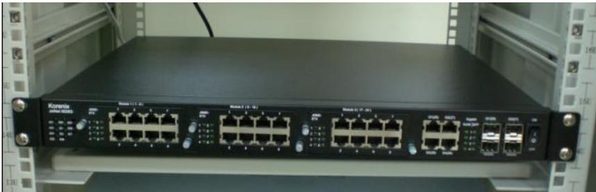
When installing multiple switches, mount them in the rack one below the other. It's requested to **reserve 0.5U-1U free space for multiple switches installing**. This is important to disperse the heat generated by the switch.
