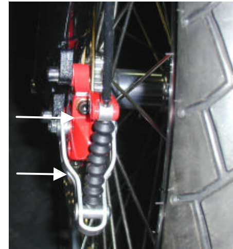
Brake Balancing: Set screws to loosen for balancing
