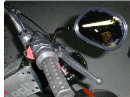
Step 19: Mirror mounted on right brake housing
