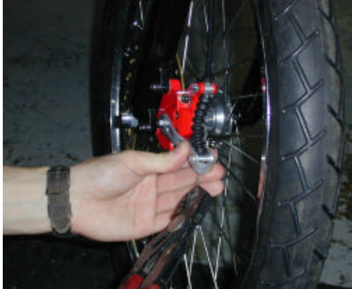
Brake Tensioning Step 2: Brake cable pulling
