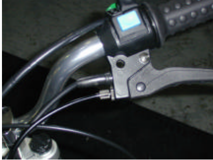
Step 15: Completed brake cable insertion
