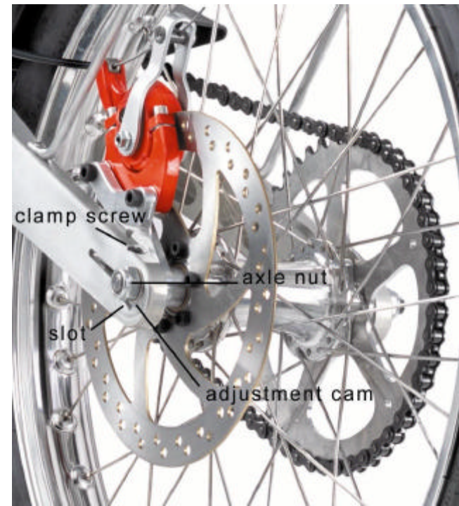
Chain Tensioning: Identifiers (above) and tension reference (below)
