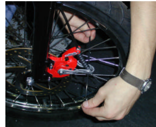
Brake Tensioning Step 1: Brake cable clamping mechanism
