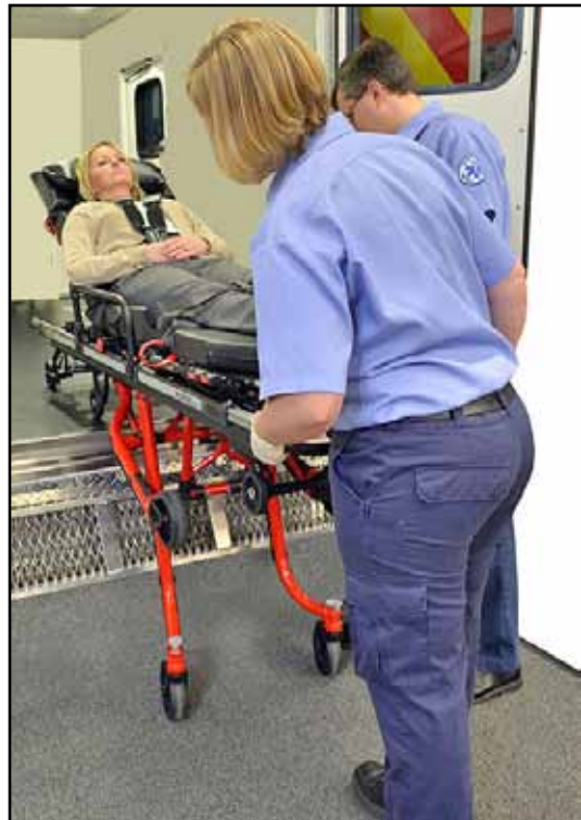
Figure 34 - Verify the Control Legs Have Locked
