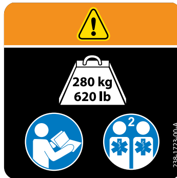
Safety Information Label (Affixed to the control panels)
