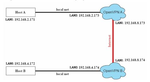
2. On machine OpenVPN A, modify the remote address in configuration file /etc/openvpn/tun.conf.
