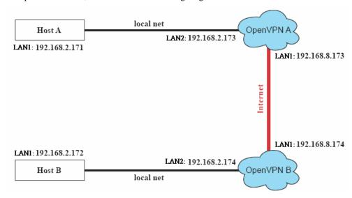
2. The configuration procedure is almost the same as for the previous example. The only difference is that you will need to comment out the parameter **up** in /etc/openvpn/tap0-br.conf of OpenVPN A and /etc/openvpn/tap0-br.conf of OpenVPN B.
