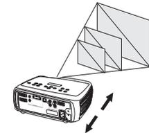
Adjust the zoom or focus rings by rotating them until the desired image size and focus are produced.
