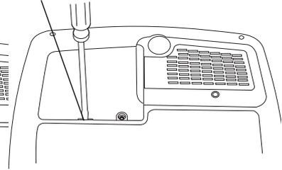
remove the screws on lamp module
