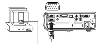
If you prefer connecting your LP640 to your computer with an optional VESA cable, connect one end of the cable to the VESA port on your computer, and connect the other end of the cable to the blue **Computer 2** connector on the projector.
