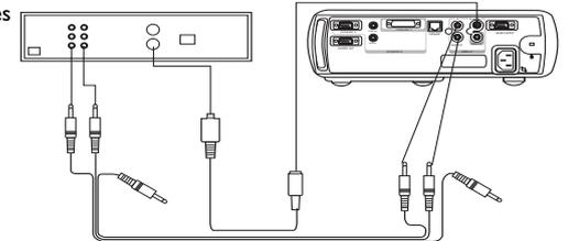
To connect a progressive scan EdTV or HD source, use the Component to M1 adapter (sold separately).
