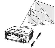
Adjust the zoom or focus rings by rotating them until the desired image size and focus are produced.
