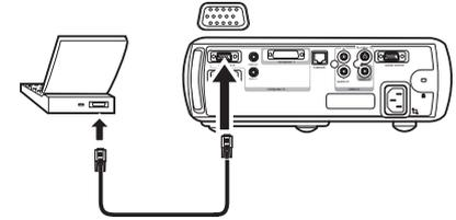
You can control the projector from an LCD control panel or computer by connecting an RS-232 cable to the projector's **Serial** connector. Specific RS-232 commands can be found in the Service and Support section of our website.
