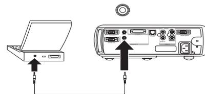
If you are using a desktop computer and want to see the image on your computer screen as well as on the projection screen, plug the monitor cable to the black **Monitor Out** connector on the projector.
