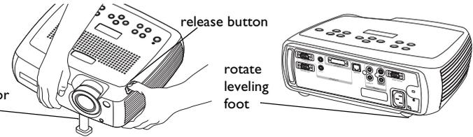
Position the projector the desired distance from the screen at a 90 degree angle to the screen. See page 42 for a table listing screen sizes and distances to the screen.
