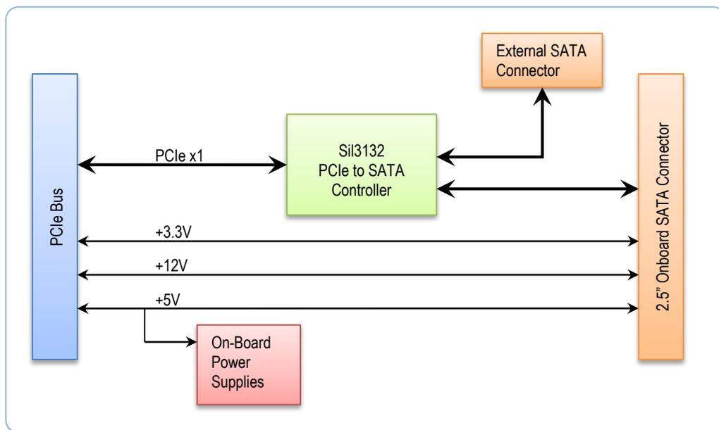
Figure 6: IOM35106 Block Diagram
