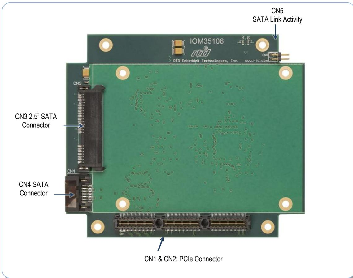
**Figure 2: Board Connections**
