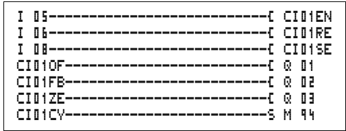
Figure 93: MFD-Titan circuit diagram with high-speed incremental encoder counter
