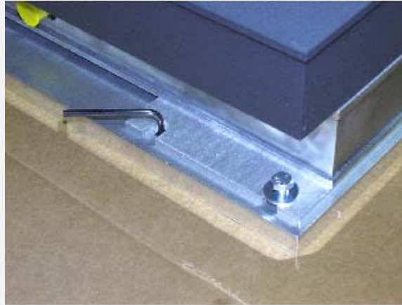
Figure 2.2 – The Mounting Plate can be leveled while the force plate is mounted on it.
