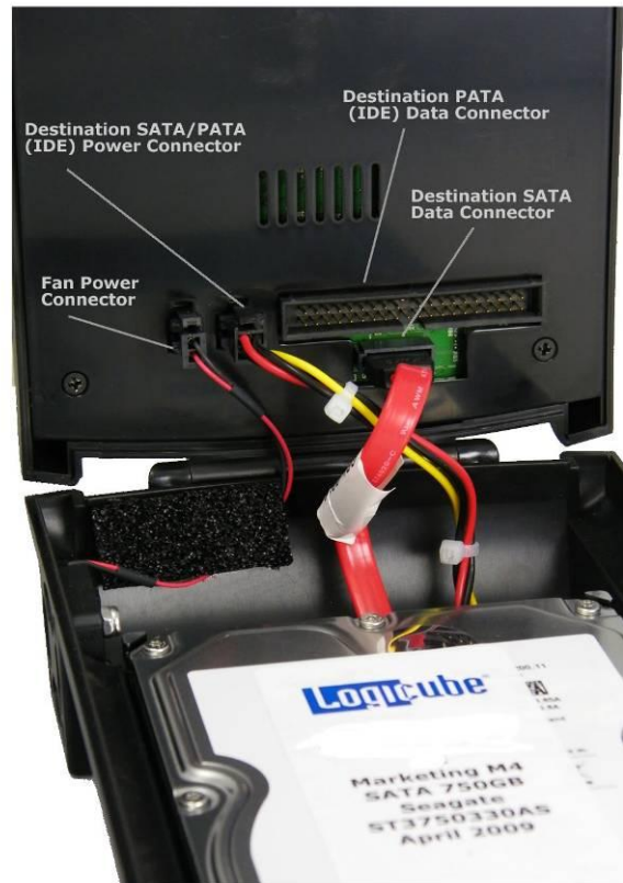
Figure 8, “Connecting SATA Destination drives to the Logicube Quest”.
