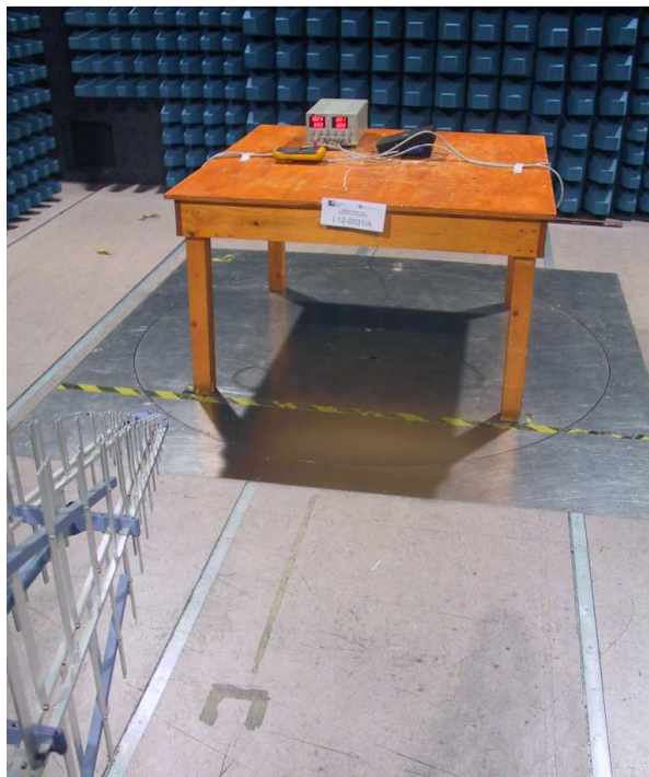
Measurement of radiated emissions
