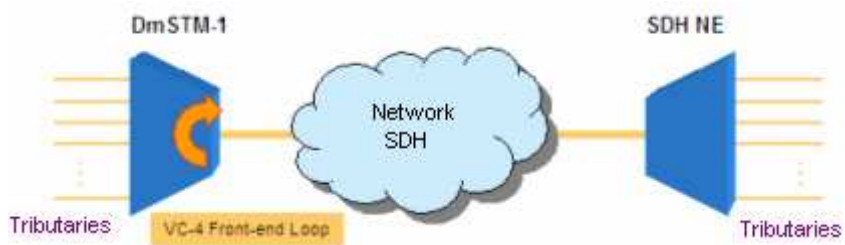
Figure 52 –VC-4 FrontEnd Loop Diagram
