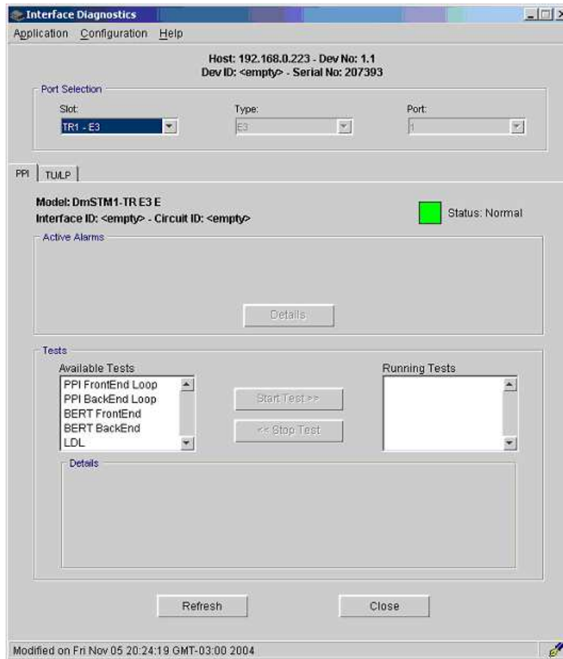
Figure 59 – Interface Diagnostics Screen for E3 Tributary PPI tests
