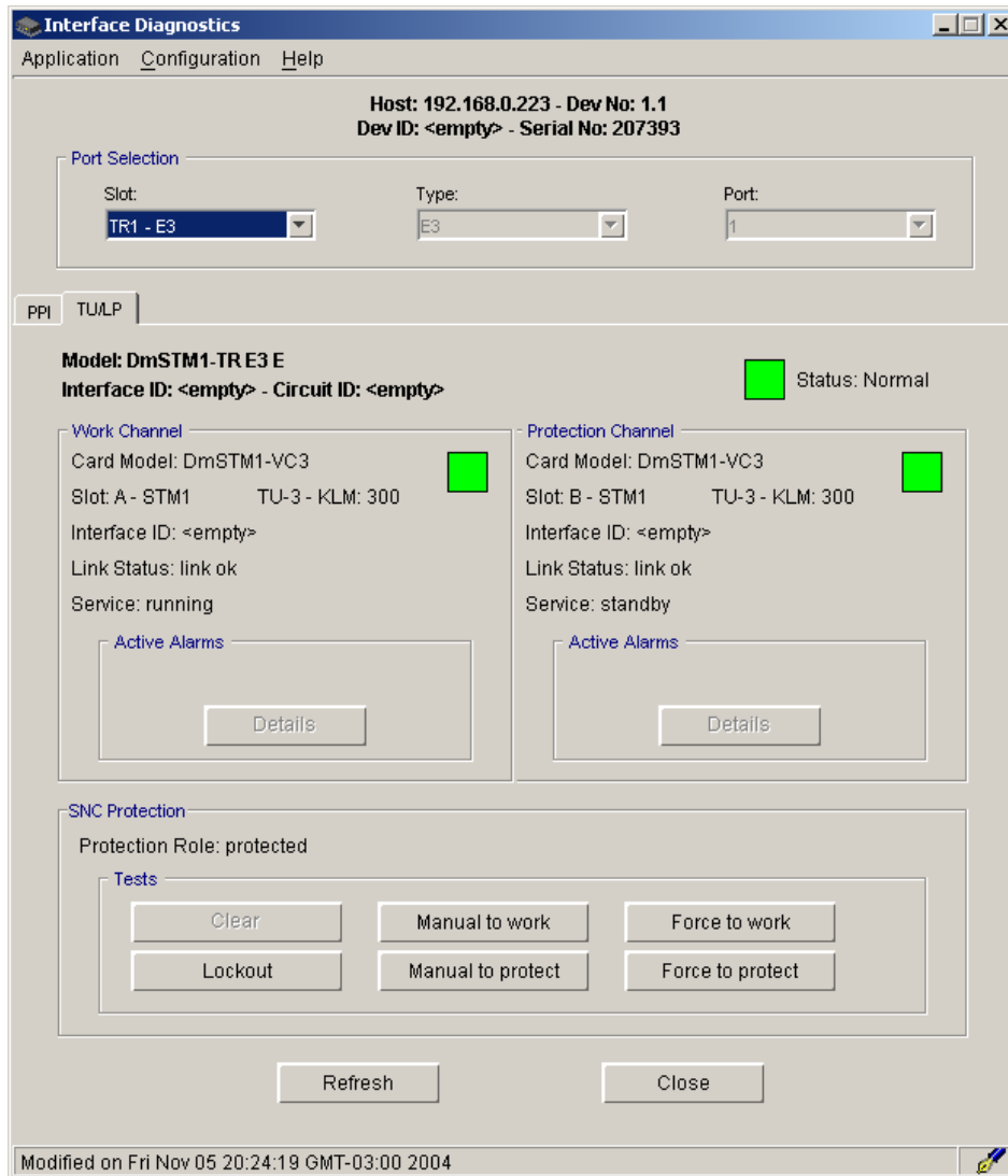
Figure 60– Interface Diagnostics Screen for SNC protection tests at the E3 Tributary
