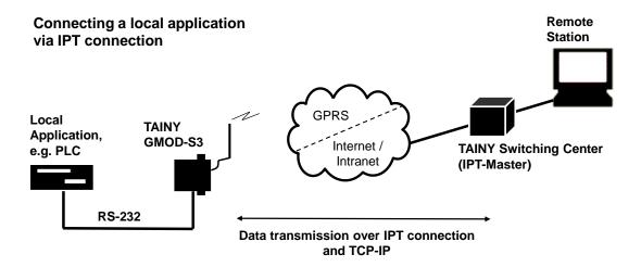
Together with the TAINY Switching Center, both dedicated connections (LL = Leased Line) and switched connections (CS = Circuit Switched) are supported by IP telemetry.
