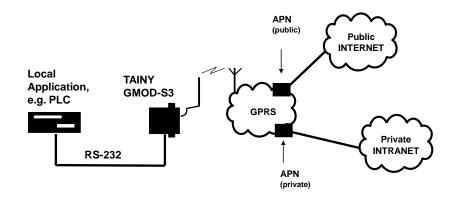
An end device that wants to establish a connection over the GPRS network indicates which network it wants to connect to by specifying the APN: internet or private company network that is connected over the dedicated connection.
