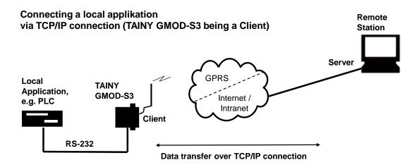
The local application and the remote TCP/IP server can exchange transparent data over the established TCP/IP connection and the local serial interface.
