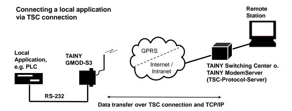
Together with the TAINY ModemServer or the TAINY Switching Center, both dedicated connections (LL = Leased Line) and switched connections (CS = Circuit Switched) are supported by IP telemetry.
