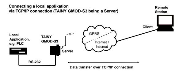
The local application and the remote TCP/IP station can exchange transparent data over the established TCP/IP connection and the local serial interface.
