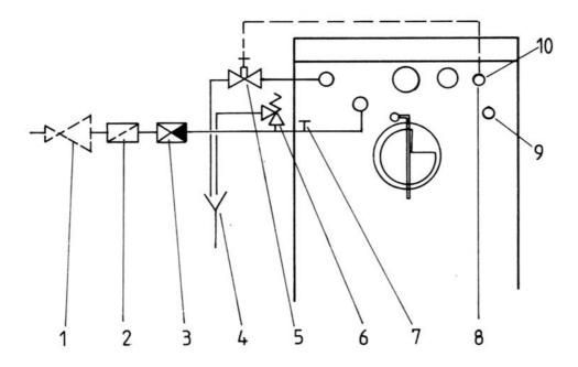
If You wish to install the boiler in closed installation system, You have to install water supply and return to water exchanger built in the boiler. There are 2 pipes form side of the boiler for connection . It is very important , that You will use special valve to realase water supply when temperature will grow up above 100 C
