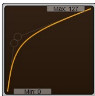
Expression Curve used to add more resolution at the top of pedal travel.
