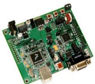
The target MCU features an on-board USB On-the-Go (OTG) physical layer (Phy). The OTG Phy may be configured for either Host or Peripheral mode depending on the target application.
