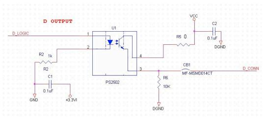
The maximum current thru the transistor should is limited to 100mA by the *CB1* fuse. User should supply *VCC* to collector of the transistor.
