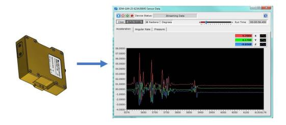
Figure 3 - Acquiring Sensor Data with MIP<sup>™</sup> Monitor
