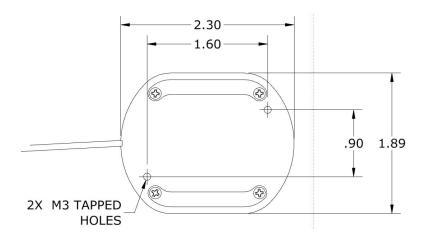
Figure 32 - GPS Antenna Mounting
