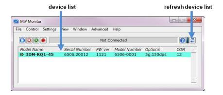
Figure 8 - Sensor Communication
