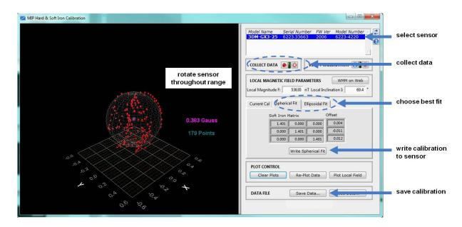
Figure 25 - Collect Calibration Data
