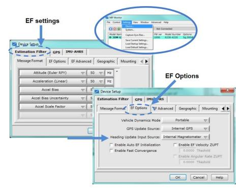
Figure 28 - Heading Source Setting
