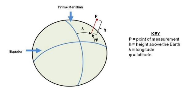
Figure 19 - World Geodetic System (WGS84) Reference Ellipsoid
