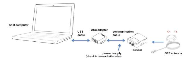
Figure 5 - System Connections
