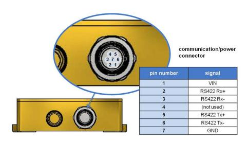
Figure 36 - Connector Wiring
