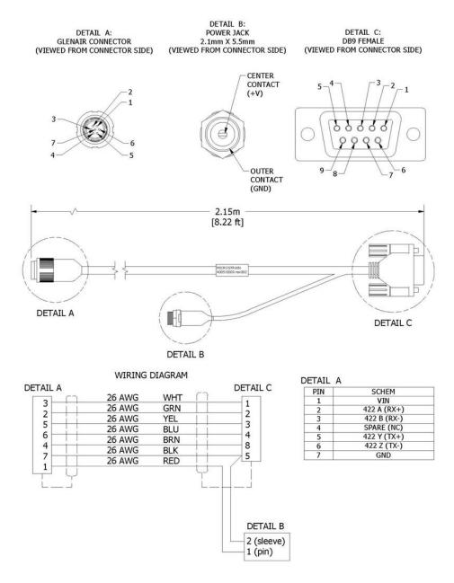
Figure 42 - Communications and power cable (PN: 4005-0009)
