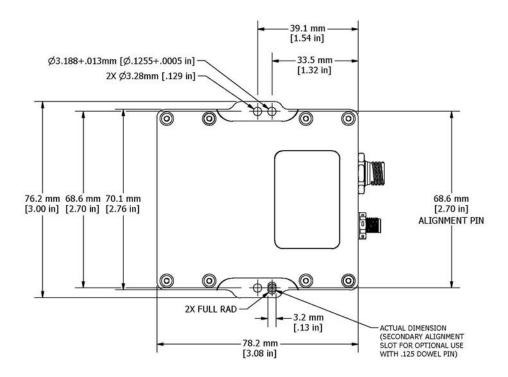
Figure 31 - Mounting the Sensor
