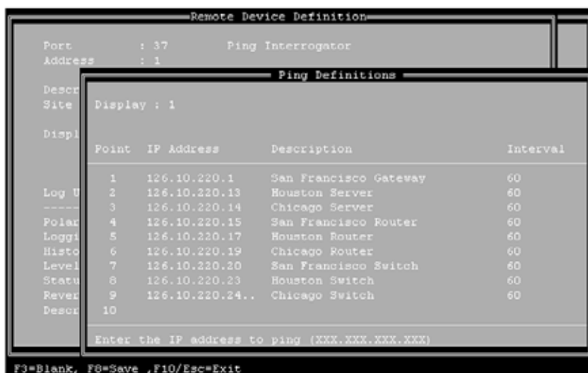
The Ping Interrogator enables T/Mon to monitor IP networks, checking to see if other network elements are present by "pinging" them.
