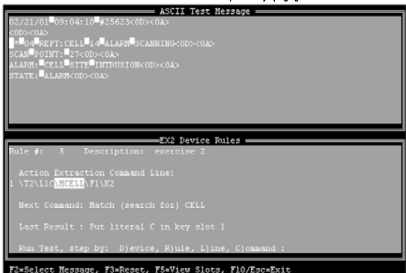
The ASCII debugger allows you to use actual ASCII alarm messages to test your rules, making ASCII rule programming much easier.
