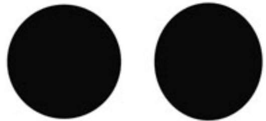
(Left) Square pixel image displayed on a computer. (Right) Square pixel image displayed on a TV.
