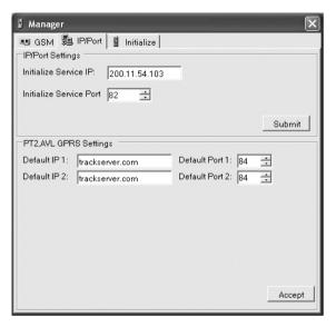
To be able to receive and send data packages from GPS/ GPRS Tracking devices over GPRS, all devices have to be configured with the IP address (or domain, if applicable) and port number used for data exchange with the Control Base Server.
