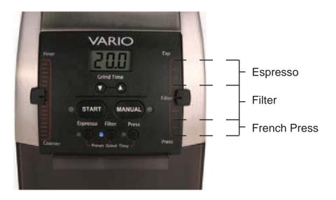
Grind a small amount of coffee by pressing the START button (Pos. 10), and then press the button again to stop the grinder. Check the fineness of the ground coffee. If the fineness is approximately to your liking, use the micro-lever for the fine fine adjustment of the grinding level. If the fineness needs to be changed significantly, prior to the next operation move the macro-lever to a new position and then make the fine setting using the micro-lever.
