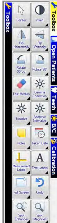
If the toolbox is not in 'locked' mode it can be customized to display the desired toolbox option. Refer to section 11.2.2 "[Customizing the Toolbox](#)" for additional information on customizing the Toolbox and the available options. To change the toolbox size, select **Tools > Toolbar/Toolbox Button Sizes**.
