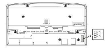
Relay connector is located under the metal back plate. Figure above shows connector position and pin assignment. Both Normally Closed (N.C.) and Normally Opened (N.O.) contacts are provided.
