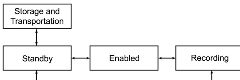
When the voice recorder is enabled, it is possible to playback recordings, set the operating parameters and connect to a PC to change the PIN-code or the protect key. Recording start/stop is possible practically in any state. Set "REC/STOP" switch (Fig. 6.1) to the appropriate position. Details of the Voice recorder operations are considered below.
