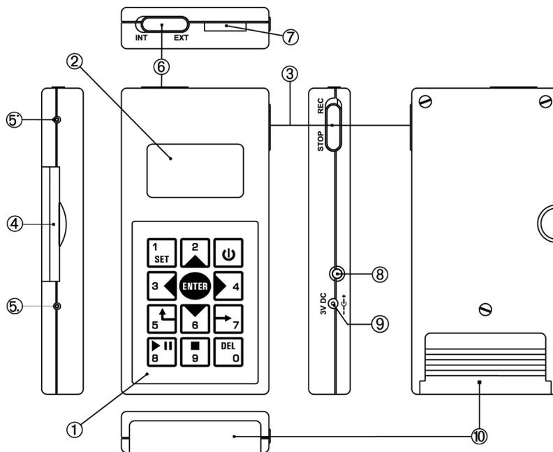
Figure 6.1: Voice recorder connectors and controls
