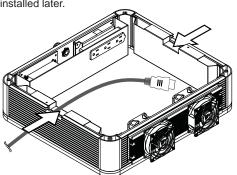
Realign the metal base plate on the Media Player Enclosure. Reinstall the 4 screws into the metal base plate while making sure the wires are fully sealed (Cables should be completely surrounded by compressible foam gaskets and gasket block).
