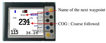
A waypoint is reached when the vehicle is in the radius defined for the wpt (200m or 90m). The GPS switches automatically to the next waypoint.
