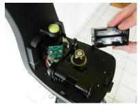
3. Once the cover is removed, take out the two AA battery compartments.
