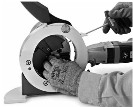
Fig 7 Installing the Tool Holder
