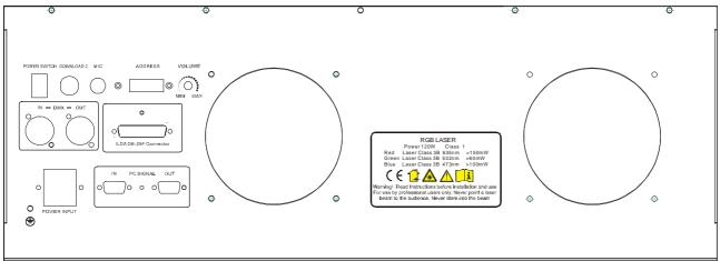
**POWER INPUT:** Input power, with inner fuse.
