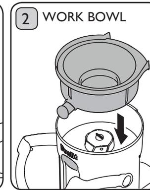
Insert the spout of the work bowl through the hole on the main body and firmly push into place.
