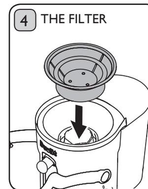
Attach the mesh filter basket by pushing it down onto the coupling of the main body until it clicks into place.
