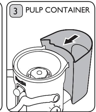
Attach the pulp container to the rear of the main body by slightly tilting and sliding it into place. **Do not operate without pulp container.**
