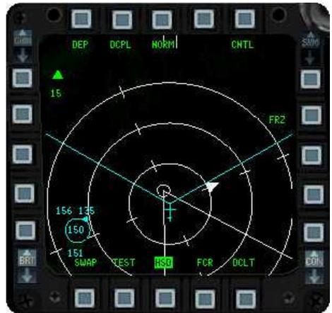
The 12, 13, and 14 OSB buttons are major mode specific. Different OSB configurations may be assigned in each major mode. These configurations will be remembered when you switch back to that major mode. There are five major modes: Navigation (NAV, the default mode), Air to Air (A-A), Air to Ground (A-G), Missile (MSL) and Dogfight (DGFT).
