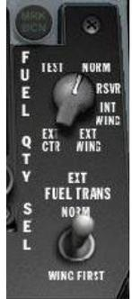
The normal fuel transfer procedure from external to internal is to transfer fuel from the centerline tank first, then from the external wing tanks. However, this may be overridden by setting the **fuel transfer switch** to WING FIRST.
