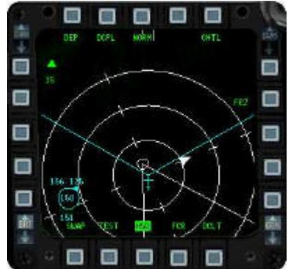
In Centered (CEN) mode, the display view centers the ownship on the MFD. Two range rings appear in this view and divide the display into equal thirds distance (rings at 5 miles and 10 miles at minimum range). The minimum range is 10 miles and the maximum range is 160 miles in this view. This mode can be used as a means to zoom the display slightly since you can get a 10-mile picture.
