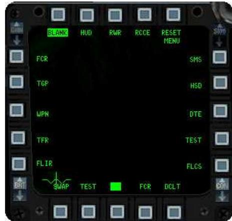
NOTE: It is not possible for both MFDs to display the same data simultaneously and therefore some MFD combinations are not possible. When attempting to display something currently displayed on the other MFD in either primary or *Secondary* buttons, the item will be 'stolen' from the MFD and replaced with a blank setting.
