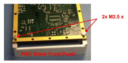
Step 2: Install the XMC module onto the VPX carrier by carefully angling the board so that the front panel slips though the gap in the metalwork. Once set align the connectors and gently push down until the connectors are fully seated.
