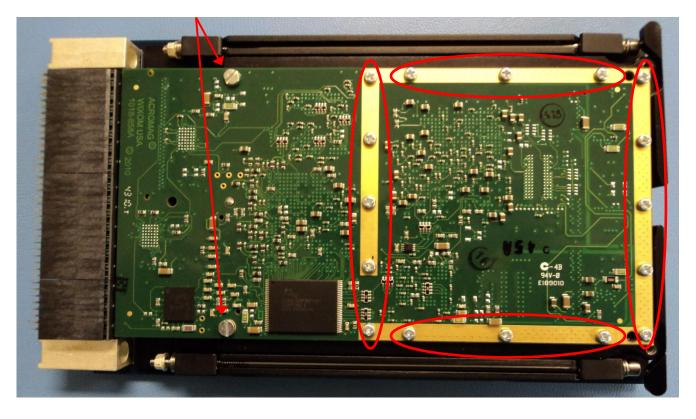
Step 5: Flip the VPX-VLX CC over and install  $2x M2.5 \times 5$  screws for the standoffs into the locations noted in the picture below. Optionally users can install another  $10x M2 \times 6$  screws into the bottom to further secure the VPX-VLX to the metalwork.
