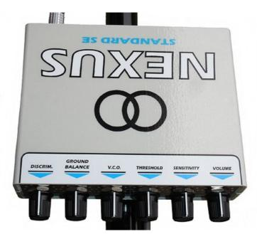
The Nexus Standard SE has seven primary control knobs and one toggle switch control. Six of the rotary controls are located on the front of the control box and the seventh is located on the back of the Meter box. The toggle switch control is located underneath the Meter box.
