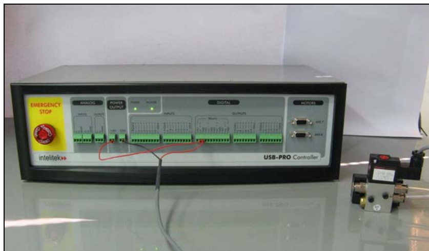
Figure 3-7: Pneumatic gripper valve connection example (front connection)
