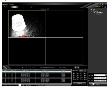
**Note:** Maximum support 4 channels when playback by time. When switching to playback from the start time, all the playback windows will be stopped and it will start playing back again.
