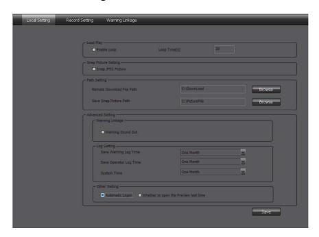
Local configuration can configure cruise in turn, screenshot, storage path, client alarm configuration, log maintenance and auto-logon option.
