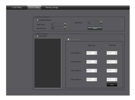
**Note:** The local recording configuration Parameters will come into effect only when the client is restarted after they are saved.
