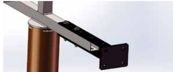
Align two (2) holes from the pattern of the Inner Headboard Bracket (A) with the two (2) holes of the square tube frame such that a distance of approximately 1.5 inches to 2 inches exists between the edge of the TEMPUR-Ergo Premier adjustable base and the Headboard Bracket assemblies.
