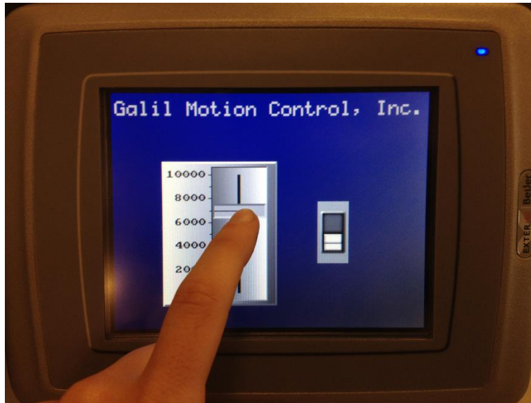
Figure 12: Using the slide to adjust the speed in counts/second
