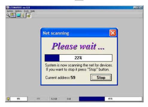
During the scanning, the program checks **Identification numbers** of recorders working in the network, trying to connect with them. The currently checked **Identification number** and a percentage of the entire scanning operation are displayed in the window. If the program connects to a device of given number, its type is being recognised.
