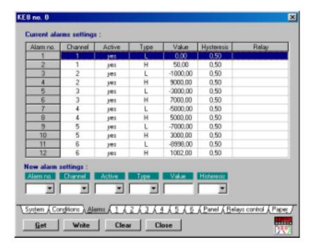
The program does not check whether set alarm parameters make sense - if they are inconsistent from recorder operation rules, the recorder will report the error while attempting to save.
