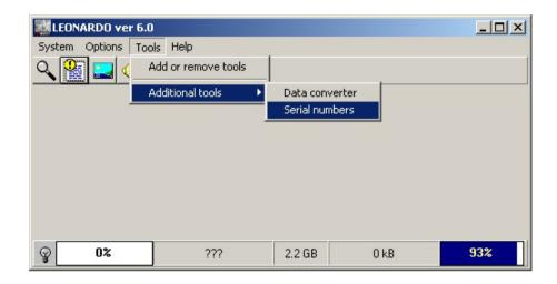
The **Data converter** program converts files containing measurement data recorded on the computer disc from recorders serviced by the **LEONARDO** program, from the program native format into \*.dbf, \*db, or \*.cvs or \*txt.
