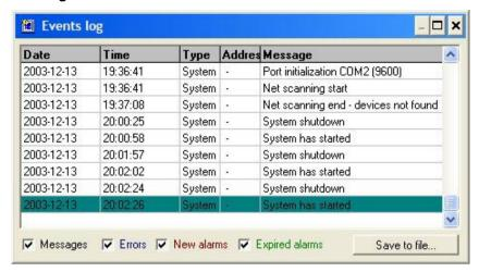
The message window enables the review of messages which occurred during the system operation. After starting the system, messages are being read from the last session with the program and one can review them by means of the scroll bar, at the right side of the window.
