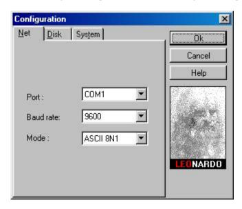
One can choose in the **Network** fold: number, baud rate and port type to which recorders are connected, the kind and parameters of the communication protocol of serviced recorders.
