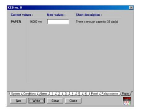
The length of paper in the roll can be programmed in the **Paper** panel writing it in the **New values** window. During the program working, the current information about the number of working days for which there is enough of paper, is currently displayed.
