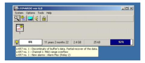
The switched on bulb signals the occurrence of events (e.g. alarms) in the recorder, the switched off bulb - a normal state of the system operation. Messages informing about events can be read out in the bulb hint, besides they are recorded in the message window together with the date and full description.
