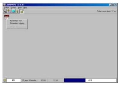
After choosing the **Parameters copying** option, the dialogue window is opened enabling the copying of chosen parameter settings from the given recorder into other recorders of the same type, e.g.:
