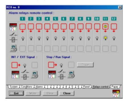
Bulbs in the middle row show the current activity of the relay (is on = active alarm), is off = inactive alarm).
