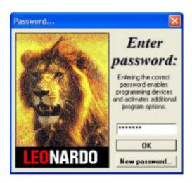
After writing the correct password in, the padlock icon in the tool bar changes into an opened padlock and remains pressed until the moment of the system protection. To protect the system again, it is sufficient to click again on Lock the system option in the System menu window of the main program. The locking and unlocking of the system is written each time in the message file, in the form of a message submitted by the system ("System" word in the Type column).
