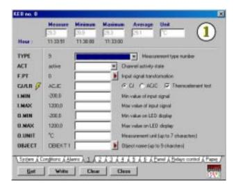
The lightning symbol CJ/LR G CJ = next to the representation of compensation kind informs, that at temperature measurements with a thermocouple the recorder tests the thermocouple break with a pulse current.
