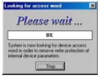
The program automatically finds the **opening word**, however it may even last up to 5 minutes, and with many recorders operating on the network, even longer. If the system has not been unlocked, the **opening word** must be entered each time while entering KE8 window.
