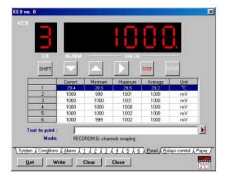
The panel duplicates the recorder display and keyboard operation.
