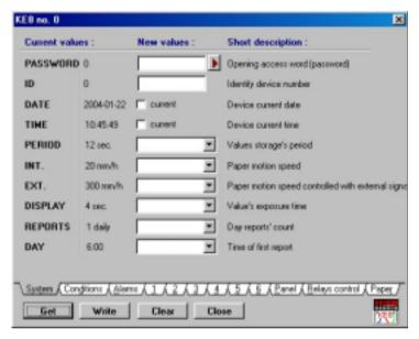
If the system of the **LEONARDO** program is unlocked (p. 5.6.) then, after pressing the key, on the right side of the edit field, the option of the automatic read-out of the recorder **Password** is accessible.
