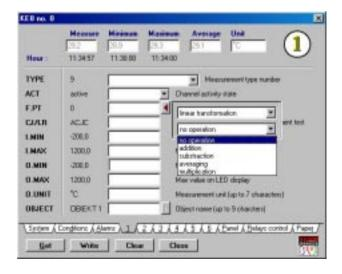
Particular options are chosen from dropdown lists, after pressing the key the window closes and selected function is inserted into FPT value field. The meaning of each option is explained by means of following hints:
