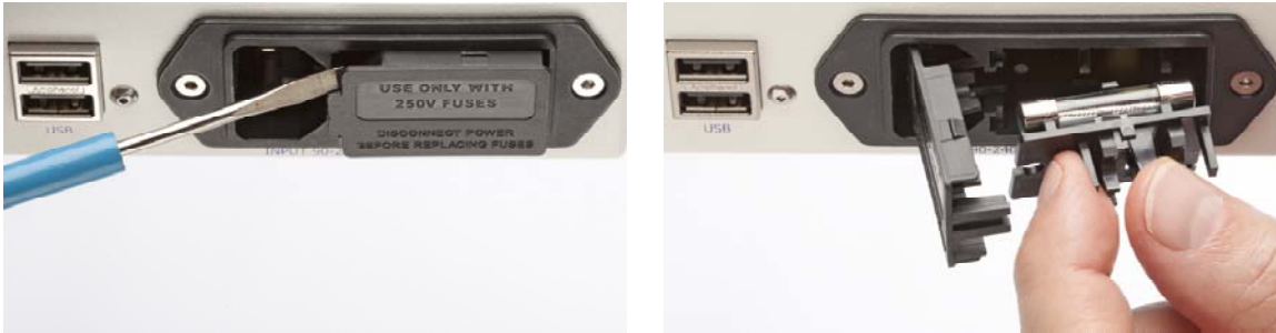
Figure 19 Replacing the Mains fuse
