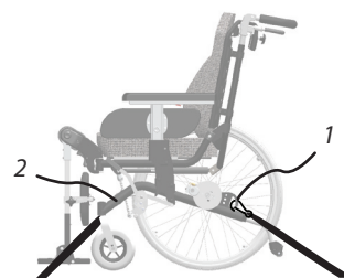
Diagram 48. Wheelchair with clamp mounted.
