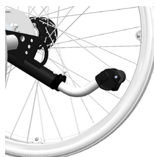
Diagram 9. Antitip device in angled position.
