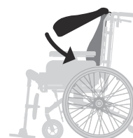
Diagram 12. Fastening straps around the flexi-frame.
