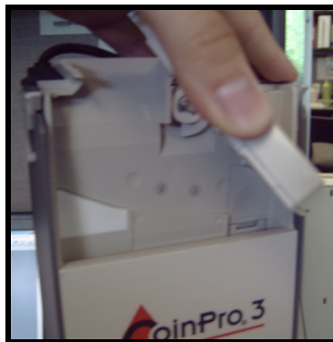
Opening the Top Portion to Expose the Sensors
