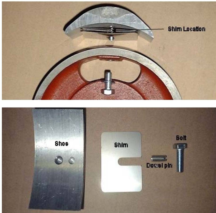
Figure 22 - Rotor Shoe Assembly & Component identification
