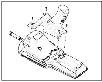
• Using a Phillips screwdriver, securely fasten the pistol grip to the back of the 7530 G2.
