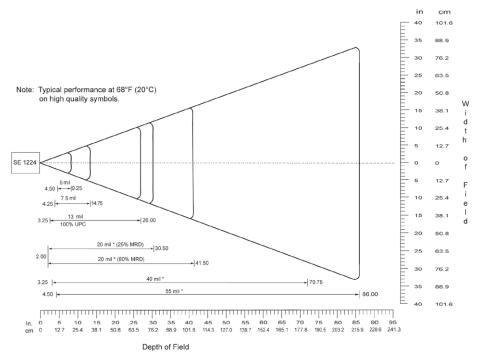
\*Minimum distance determined by symbol length and scan angle
