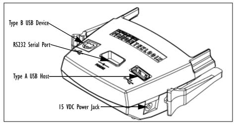
Figure 6.2 PDM Ports And Connectors
