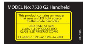
Figure 1.4 LED Radiation Notice Label
