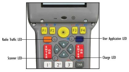
Figure 3.3 Keyboard LEDs
