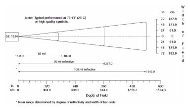
Figure 7.2 I524ER Decode Zone B (long-range, large codes)
