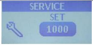
Use the Up and Down Arrow buttons to select the desired number of service cycles. The press the Menu button to lock in this value and return to Menu screen #2.
