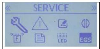
With the large wrench icon displayed and the word SERVICE showing at the top of the screen, press the Menu button.
