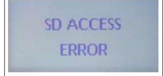
If you have not plugged in the SD Card reader or the SD card is not inserted into the Reader, this message is displayed and then Menu screen #2 is redisplayed.
