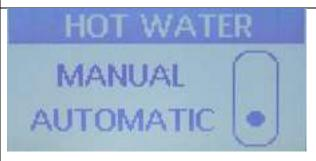
This screen will display the current setting. Use the up or down arrows to select the MANUAL or AUTOMATIC setting, then press the Menu button. If you selected Manual, you go back to the main profile menu. Manual means that you press the Hot Water button to turn it on and press it again to turn it off; i.e. manual operation.
