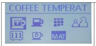
Starting from the last menu in the previous section, press the Down arrow to highlight the Coffee Temperature icon and display COFFEE TEMPERAT on the top of the screen. Then press the Menu button to enter the Coffee temperature (group boiler) programming screen.
