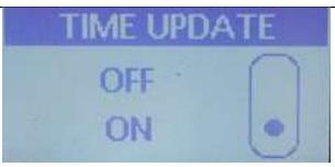
Use the Up or Down arrows to select either OFF or ON and then press the Menu key to lock in the selected value. If OFF is selected there will be no automatic Daylight Savings time adjustment. If On is selected you are taken to the next screen to pick your desired option.
