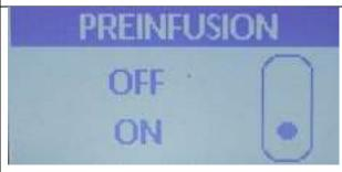
Use the Up or Down arrow to select whether preinfusion is on ON or OFF, then press the Menu button. If OFF was selected you immediately return to the main Profile menu and you have no preinfusion on either the One Cup or the Two Cup button.
