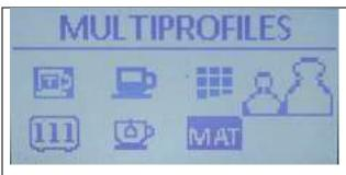
Depending on where you are in the profile menus, press the Up or Down arrow to highlight the Multiprofiles icon and display that text on the top of the screen. Then press the Menu button to enter the MULTIPROFILES programming screen.
