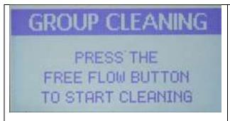
Press the Continuous Flow button (the one between the One-Cup and Two-Cup buttons) to begin the cleaning operation. It continuously cycles 5sec On / 5sec Off.
