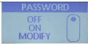
Use the Up or Down Arrows to select the desired password mode. If you do not want the configuration menu to be password protected set this to OFF. If you want the password protection feature, turn this setting ON to use the current password. If either of these options is selected, pressing the Menu key locks in that value and returns you to Menu screen #3. Selecting Modify and then pressing Menu takes you to the next screen.
