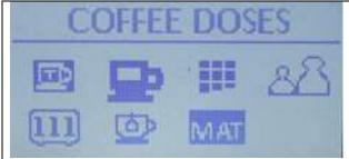
Depending on where you are in the profile menus, press the Up or Down arrow to highlight the Coffee Doses icon and display that text on the top of the screen. Then press the Menu button to enter the coffee doses (water volume) programming screen.
