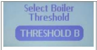
Start with the machine OFF and then press and hold the Menu button. The screen will indicate the currently set value. If it is correct you can press Menu to relock that value and exit back to the OFF state.
