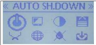
With the large On/Off button icon displayed and the word AUTO SH.DOWN showing at the top of the screen, press the Menu button.
