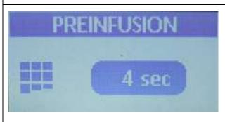
On this screen you select the number of seconds you desire for preinfusion. The value selected here indicates the number of seconds during the shot that the water is turned on running into the PF at street pressure before the pump is turned on. The amount of water programmed when you set the coffee doses is not impacted by the value used here since the total shot volume is measure by impeller turns any time the water is flowing.
