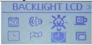
Wherever you currently are in the menu system be sure you are seeing Menu screen #1. Use the Arrow keys to get there and then highlight the Backlight LCD Time-out icon which looks like a flashlight bulb. Then press the Menu button to get into the backlight set up screen.
