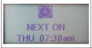
When the machine is OFF and the Programmable On/Off Timer is Enabled and On/Off times have been set, the screen shows the next ON time.
