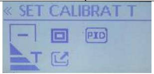
With the large Triangle T icon displayed and the word SET CALIBRAT T showing at the top of the screen, press the Menu button.
