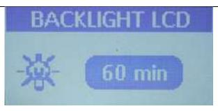
This setting adjusts the amount of time the display stays backlit after that last front panel button press. The maximum is 60min which is shown on the display. The options are 5, 10, 30, or 60 minutes. Use the Up and Down Arrows to select your desired option, then press the Menu button to lock in the value and return to Menu screen #1.
