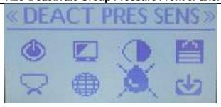
With the large "Drop with and X through it " icon displayed and the word DEACT PRES SENS showing at the top of the screen, press the Menu button.
