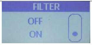
Use the up or down arrow buttons to select OFF or ON, then press the Menu button to activate your choice. If OFF is selected, the previous Menu screen #2 is displayed. In this case you will received on Filter replacement notification. If ON is selected you are taken to the next Menu Option.
