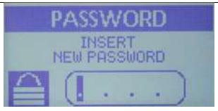
Next use the Up and Down arrow keys to scroll through the choices for the 1<sup>st</sup> character. Only the numbers 0-9 are available and only four characters are used so this is really a PIN number more so than a password.
