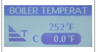
The Owner's Manual instructs that this value should only be changed by a trained technician. Apparently this can correct for inaccuracies of the steam boiler temperature sensor. However, the steam boiler temperature is only selected in order to adjust for the desired steam pressure. Therefore, knowledge of the absolute temperature of the boiler is not really required.
