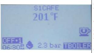
Note that the word OFF in the lower left corner of the display is followed by +1 in this photo. This means that the time listed below OFF+1 is for tomorrow. If the display only showed OFF the time below would be for today. (This is the same as OFF+0!) OFF+2 indicates the day after tomorrow and so on. There are two ways to interpret this timer status display which require that the user know how the machine was last turned on.
