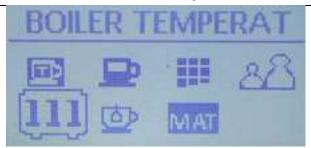
Depending on where you are in the profile menus. press the Up or Down arrow to highlight the Boiler Temperature icon and display BOILER TEMPEARAT on the top of the screen. Then press the Menu button to enter the boiler temperature (steam boiler) programming screen.
