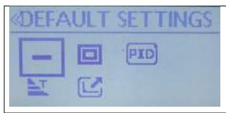
With the "Large Square with a line in the middle" icon displayed and the word DEFAULT SETTINGS showing at the top of the screen, press the Menu button.
