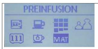
Depending on where you are in the profile menus, press the Up or Down arrow to highlight the Preinfusion icon and display that text on the top of the screen. Then press the Menu button to enter the programmable preinfusion programming screen.
