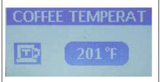
Use the up or down arrows to increase or decrease the indicated temperature until the desired espresso temperature is showing.
