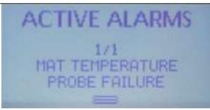
If you have a triangular alarm icon in the middle of the Home Screen and you navigate to this page, you will see the text of the alarm. If there are more than one active alarm you can use the Up and Down Arrows to scroll back and forth through the active alarm list.
