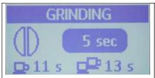
Use the Up or Down arrows to scroll to the desired value. As you can see from this and the next two screens the options are 5, 10, or 15 seconds. The value initially displayed is this last value that was set for this feature.
