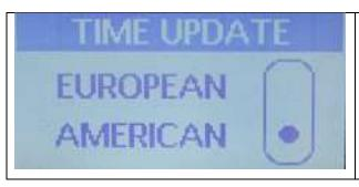
Use the Up or Down arrows to select either the European or the American Daylight Savings time Start/Stop dates. Then press the Menu button to lock in the value and return to Menu screen #3.
