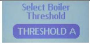
If you need to change to the other threshold value use the Up or Down Arrow keys to display it and then press the Menu button to return to the OFF state.
