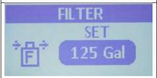
Use the Up and Down Arrow buttons to select the desired number of gallons of water that you can run through your filter. The press the Menu button to lock in this value and return to Menu screen #2. Note that since the Tank model only supports a small in-tank filter the range for this setting is much smaller than on the plumbed models.
