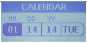
Initially, the month is highlighted. Use the Up and Down arrows to select the desired month. Then press the Menu button to lock in this value and move to the day field. Once again use the arrow keys to select the desired value and lock it in with the Menu button. Then repeat again for the Year field. When the Menu button is pressed after setting the Year, Menu screen as shown in paragraph 5 is redisplayed.
