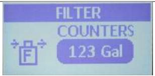
As with the Service option described previously, the initial display shows the current gallons remaining based on the last programmed count. The current filter count is also available on the status screens shown in paragraph 6. You normally only enter this menu option when you want to reset the value. If you don't want to reset the current value, one option is to step away until the screen times out and returns you to the Home screen. For the other option see the last screen in this paragraph.
