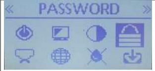
With the large Padlock icon displayed and the word PASSWORD showing at the top of the screen, press the Menu button.
