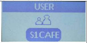
With the Home Screen displayed, press and hold the Blue Down Arrow until the Profile Menu is displayed as shown at left. Then you can use the up and down arrows to select a different profile, if you have more than one configured. With the desired Profile highlighted press the Menu button to select it, the display then jumps back to the Home Screen.
