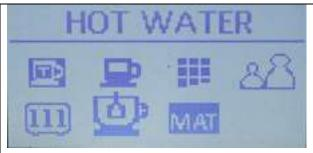
Depending on where you are in the profile menus, press the Up or Down arrow to highlight the HOT WATER icon and display that text on the top of the screen. Then press the Menu button to enter the hot water (hot water volume) programming screen.
