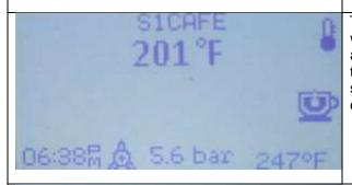
This photo shows a thermometer like icon the upper right corner which indicates that the steam boiler is refilling. (Perhaps this icon is actually supposed to be a vertical boiler!) The pump icon between the group pressure and the time is also on as it is when pulling a shot. This is how you can tell the difference between the pump being on for a shot and the pump engaging to refill the steam boiler.
