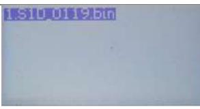
Next the Dream display lists all .bin files it has found on the card. Use the Up and Down arrows if you have multiple .bin files in order to highlight the correct one, then press the Menu button.
