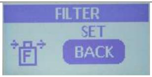
Screen values for the Plumbed version are: 1250, 500, 250, 125, and BACK. If you press BACK no new value is selected and the current value is not reset. If the current value and the selected value are the same the menu does not show the BACK option. If, for example, you reset the value to 125 Gal, exit the filter menu, then come right back in, you will not see a BACK option since the set value and the current value are still the same.
