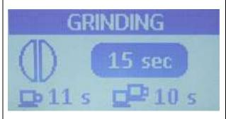
Assume that the programmed dose time is 25 seconds and that the GRINDING value is set to 5 seconds.
