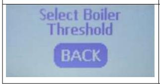
In addition to being able to use the arrow keys to display Threshold A or Threshold B you can also scroll until BACK is displayed, pressing Menu with BACK display returned the machine to the OFF state without changing the original threshold value.
